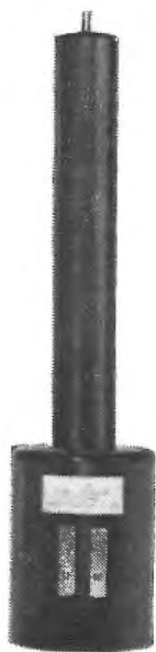
150 kV spiral generator from Wego Condenser Company.
